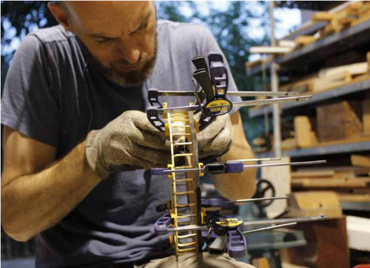
Figure 15: Coaxing together a brass stretcher plate and a buffalo leather diaphragm. Both pieces are strategically laser cut to allow certain areas to exhibit weakness, facilitating assembly, and other areas cut to gain strength from changes in geometry. With time the entire assembly
