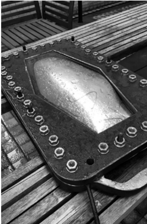
Figure 1 (top, opposite page): Early free-pressure forming test. This test successfully removed welding from the workflow, a desirable change for application to galvanised, anodised, or otherwise pre-coated metals that make welding dangerous or impossible. However, the through-bolted attachment flange on the rear of this test is not removable without destroying the final fabrication. Source: author .
