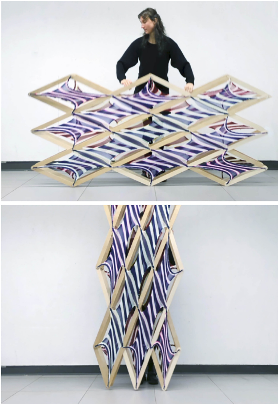
Figure 5 (this page and next). Different states of deployment of the diagonal design scissor grid.
