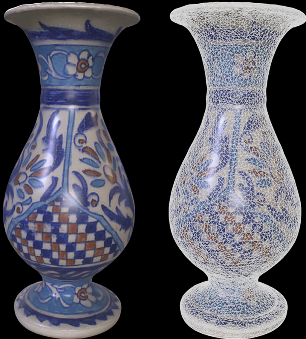
Figure 1. Example output from the workshops: High-poly model polycount: 44338 (this page). Low-poly model count: 2594 (next page). Source: Authors.
